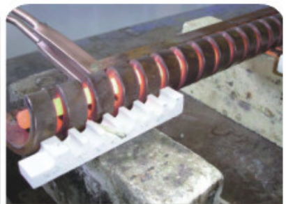
圓長棒熱鍛 Bar heating for forging
