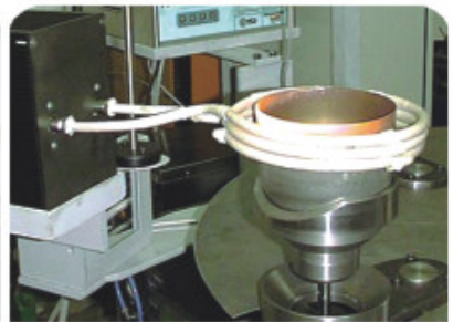
回火裝置 Annealing operation
