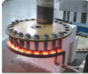
螺絲熱處理 Hardening for screws
