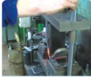
加熱壓曲 Heating for bending
