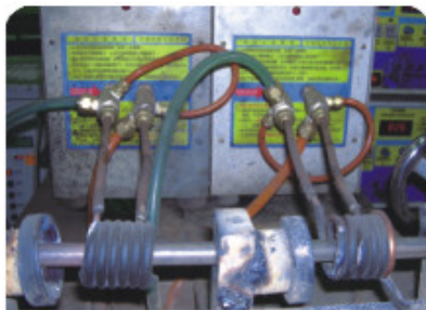
二機加熱線材 Two heaters in one line
