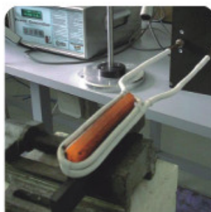
打石工具硬化 Cutting tool for stones
