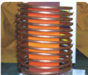
石墨鉗鍋加熱 Heating for carbon crucibles
