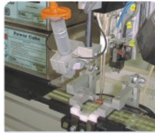
電路板以錫膏自動錫焊 Auto soldering by paste
