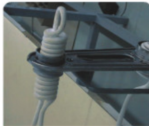
內孔加熱 Heating for insert
