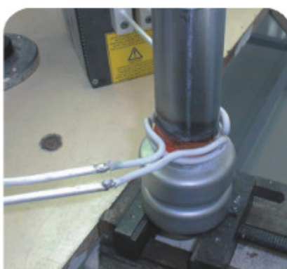
雙感應線圈同時加熱 Twin coils for one piece
