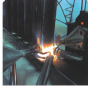
雙感應線圈同時加熱 Twin heating heads for one piece
