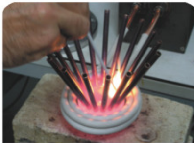
多鋼管一次焊接 Tubes soldering at the same time
