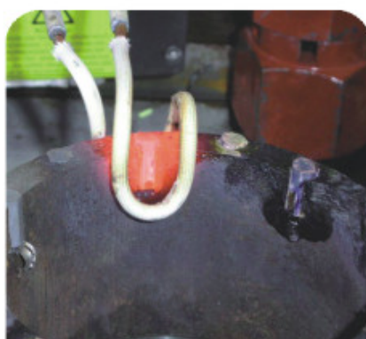
水泥鈦具焊接 Carbide tipped for circular drill
