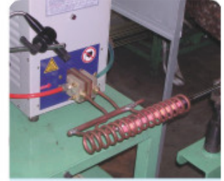
鋼筋條棒加熱鍛造 Heating for pressing
