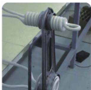
內孔加熱 Heating for insert
