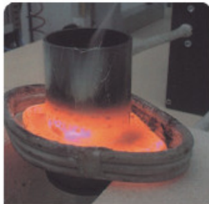
較大物件焊接 Soldering for big pieces
