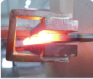
連續加熱鍛造 Continues heating for forging
